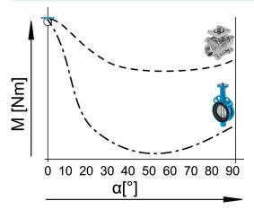
Torque required to overcome the static friction of the process valve.
