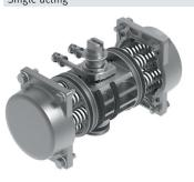
With the single-acting quarter turn actuator, the incoming compressed air moves the pistons in one direction. This generates the torque of the actuator. At the same time, the springs built into the actuator are pre-tensioned. This spring force generates the torque in the opposite direction of rotation when the pressure chambers of the actuator are exhausted. This causes the angle seat fitting to move to the required initial position.
