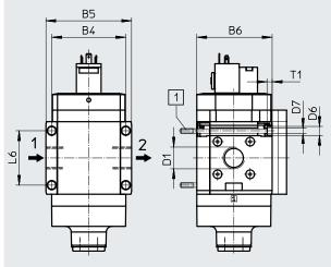
[1] Retaining screw M6xmin. 90 to DIN 912 (not in the scope of delivery) for wall mounting without mounting bracket Flow direction
