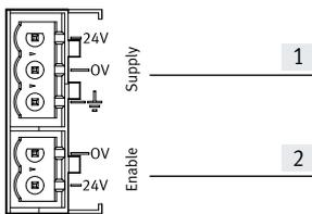
The valve terminal has a connection for the power supply for electronics and valves [1].
