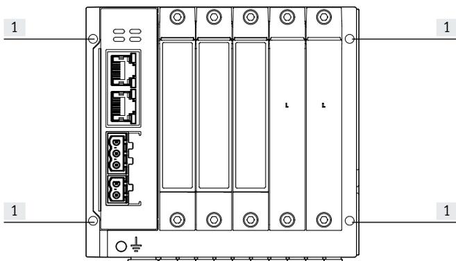
The manifold sub-base has four through-holes [1] for mounting the valve terminal.
