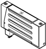
VTEP offers two different valves, one for high pressure and one for low pressure. The valves comprise four 2/2-way proportional valves connected to form a bridge circuit, two of which regulate the pressure in duct 2 and two of which regulate the pressure in duct 4.
