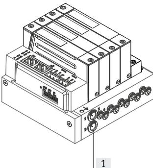
The valve terminal VTEP is supplied with pressure via the connections [1] in the manifold sub-base.
