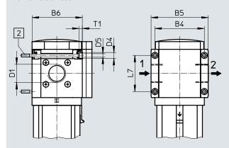
[2] Retaining screw M6xmin. 90 to DIN 912 (not included in the scope of delivery) for wall mounting without mounting bracket
