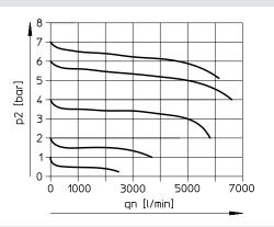
Pressure regulation range 0.5 ... 12 bar  $\,$  Grade of filtration 5  $\mu m$  MSB6-1/4
