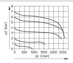
Pressure regulation range 0.5 ... 12 bar  $\,$  Grade of filtration 5  $\mu m$  MSB4-1/8
