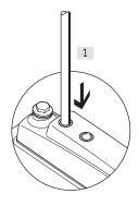
[1] Press in the plunger of the MO with a blunt plastic pin.The pilot valve switches and actuates the main valve.
