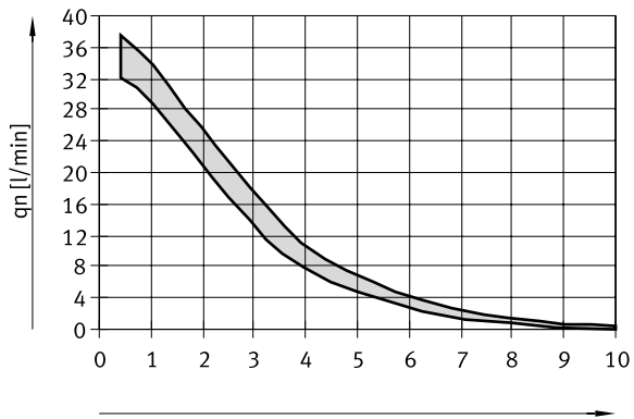
Standard flow rate q_n at 1 → 0 bar as a function of spindle rotations n (Size 160)
