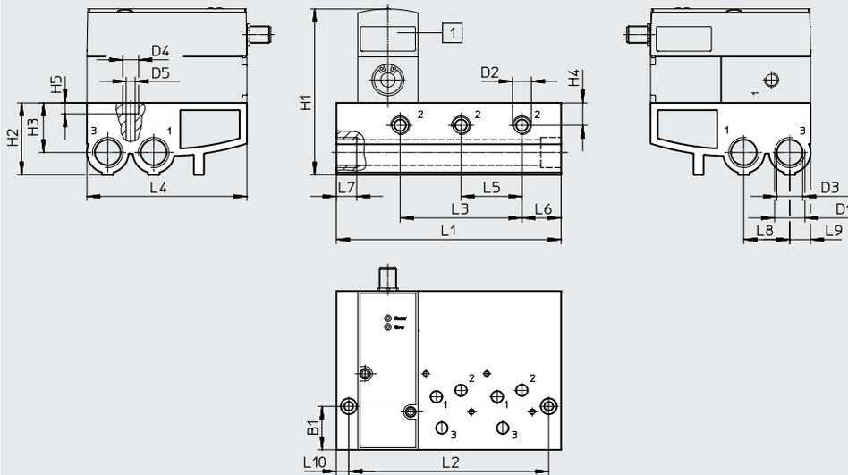
[1] Proportional-Druckregelventil VPPX
