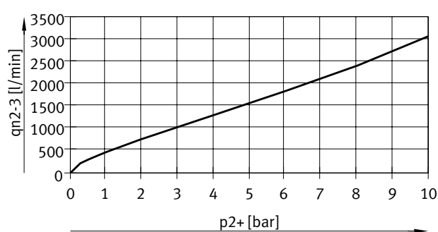
Flow rate q_n from 2 > 3 as a function of output pressure p_2
