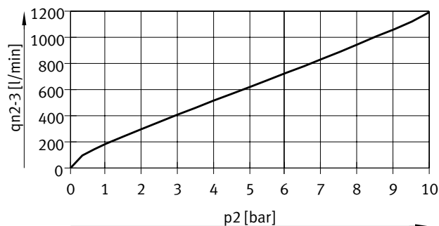
Flow rate q_n from 2 > 3 as a function of output pressure p_2
