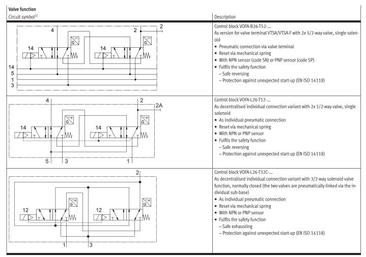
1) The symbol represents a valve with a proximity switch with a switching output signal, in the illustration an N/O contact. In line with ISO 1219-1, this symbol applies to both N/O and N/C contacts. The switching element function of all sensors used here is an N/C contact.
