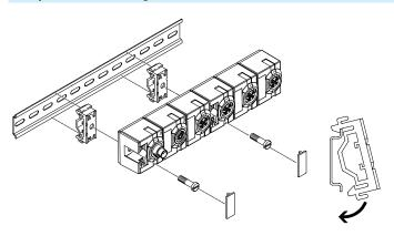
The base for H-rail mounting is screwed onto the component and the entire unit can then be placed on an H-rail. Depending on the product, mounting holes can be covered by inscription labels.
