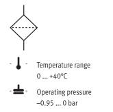
The vacuum filter is used to filter particles in the suction direction.
