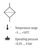
The vacuum filter is used to filter particles in the suction direction.
