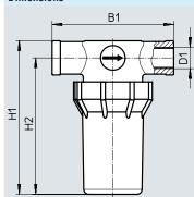
Ordering data Connection В1 Н1 Weight Part no. H2 Туре [g] 1/4 71 547261 VAF-DB-1/4 94.5 84.5 75 3/8 90.5 125 113 156 553140 VAF-DB-3/8 1/2 90.5 129 115 162 553141 VAF-DB-1/2
