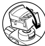
Turn MO to clip it onto the pilot valve. The MO cap can then be operated (detenting) without tools. Valves can be ordered with a fitted cover cap in the valve terminal configurator using the selection menu “Manual override” (code N).
