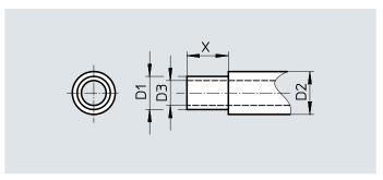
Before the plastic tubing PAN-VO can be inserted into the push-in fitting QS-VO, the tubing's PVC sheath must be cut by length X.
