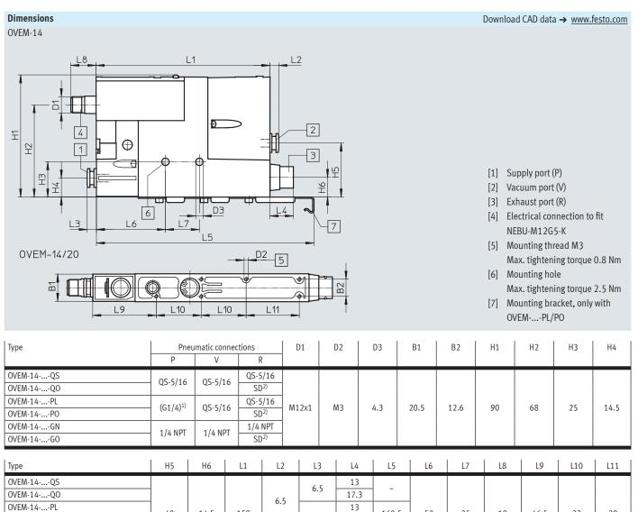
1) Thread for mounting on the common supply manifold ( $\rightarrow$  page 18)
