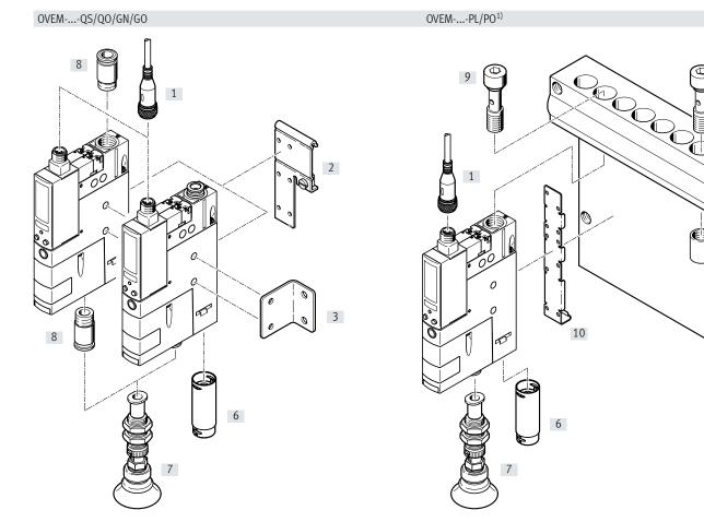
1) Hollow bolt [9] and mounting bracket [10] are included in the scope of delivery for the OVEM-...-PL/PO.
