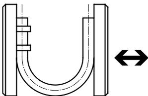
The tube fixed to the base plate is bent until the deformation results in a kink. The measured value is the minimum bending radius  $R_{min}$ . This  $R_{min}$  results in significant reductions in flow rate.
