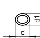
Cross-section flattened by bending the tube.
