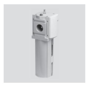
The proportional lubricator adds a precision adjustable quantity of oil to the compressed air stream. The pressure drop that occurs when air flows through a Venturi nozzle is used to convey oil from the container to the drip cap. From here, the oil drips into the air duct directly behind the proportional valve, where it is atomized. The oil mist component is proportional to the compressed air flow rate.
