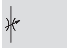
Flow control acting at both sides GRLO
