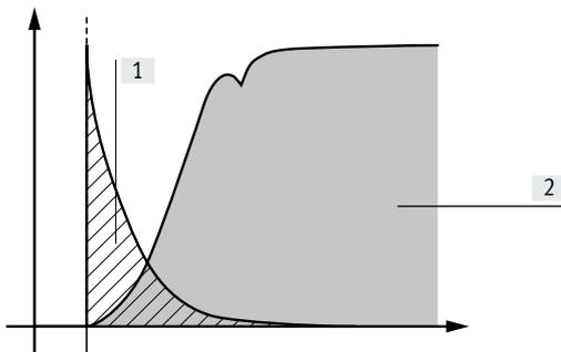
Compared with solenoid valves, proportional valves with piezo technology require virtually no energy to maintain an active state thanks to their capacitive principle. The piezo valve operates like a capacitor: it needs current only at the start in order to charge the piezoceramics.
