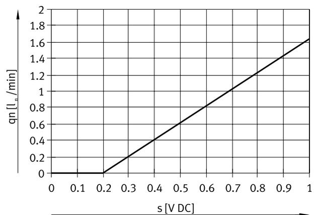
Formula for calculating the setpoint value  $s$  as a function of the required nominal flow rate
