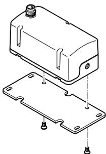
The valve VEMD is mounted on the wall mounting VAME-P14-W using two screws.
