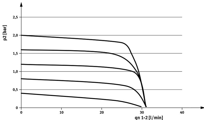
Flow rate  $q_n$  from 2 → 3 as a function of output pressure  $p_2$
