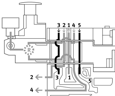
This pressure regulator regulates the pressure in duct 4 after the pressure medium flows through the valve. During exhausting, the air flow in the valve is exhausted from duct 4 to duct 5 via the pressure regulator.
