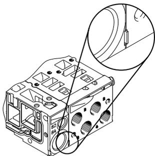
MPA offers a number of options for creating pressure zones if different working pressures are required. Depending on the electrical interface, up to 16 pressure zones are possible. A pressure zone is created by isolating the internal supply ducts between the sub-bases using an appropriate separating seal or using a separator that is permanently integrated in the sub-base (code I or code III).
