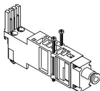
The individual compressed air supply of a single valve with a width of 20 mm can be realised using the vertical pressure supply plate VMPA2-VSP- ....
