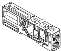
When there is a need to increase the air supply, additional supply plates can be provided.
