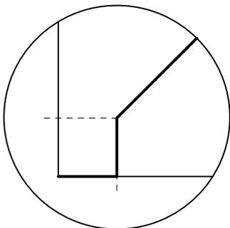
In practice, there can be a residual voltage or residual current at the setpoint input of the VPPM via the setpoint generator. Zero point suppression is used so the valve is reliably exhausted at a setpoint value of zero.
