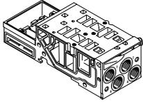
MPA is based on a modular system consisting of sub-bases and valves. The sub-bases are screwed together, thus forming the support system for the valves. They contain the ducts for supplying compressed air to and exhausting the valve terminal as well as the working
