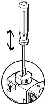
MO is actuated by pushing it with a pointed object or screwdriver and reset by spring force (detenting position prevented by coded cover cap). Valves can be ordered with a fitted cover cap in the valve terminal configurator using the selection menu “Manual override” (code N).
