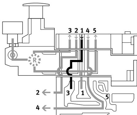
The reversible B regulator splits the supply air in duct 1 and regulates the pressure upstream of the valve in duct 3 (the unregulated pressure from duct 1 is in duct 5). The regulated air is then routed to duct 2. The valve is thus operated in reverse mode.
