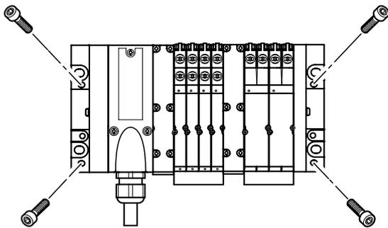
The MPA valve terminal is screwed onto the mounting surface using four M4 or M6 screws. The mounting holes
