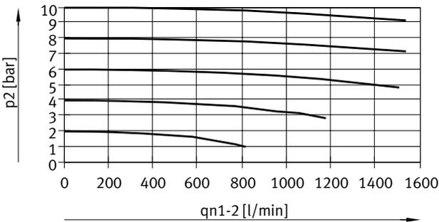
Flow rate  $q_{n2-3}$  as a function of output pressure  $p_2$
