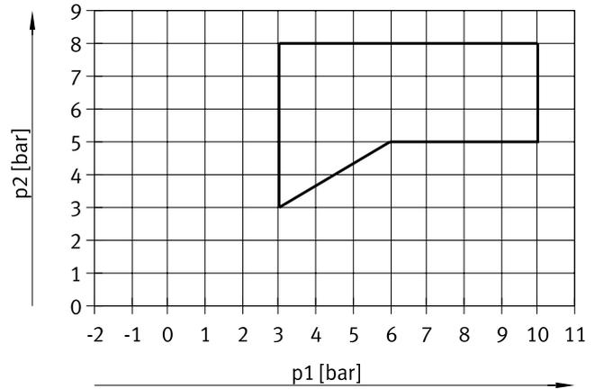
**Pilot pressure p2 as a function of working pressure p1 for valves with mechanical spring return**
