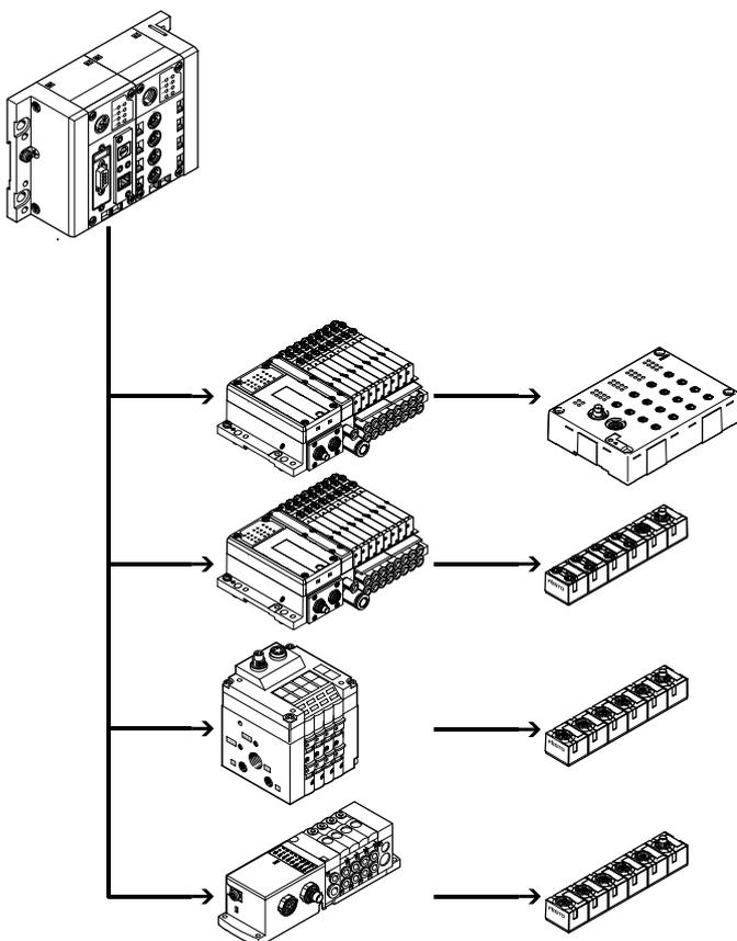
Valve terminal for installation system CPI:
