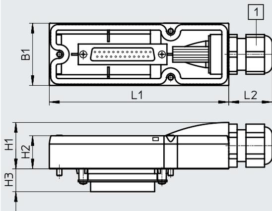
[1] Cable connector with clamping range 6 ... 12 mm
