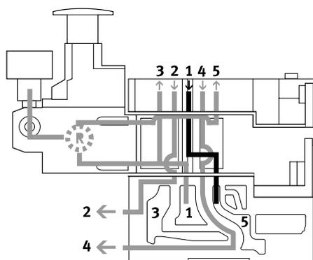
The reversible A regulator splits the working air in duct 1 and supplies the pressure upstream of the valve into duct 5 (the unregulated pressure from duct 1 is in duct 3). The regulated air is then routed to duct 4. The valve is thus operated in reversible mode.
