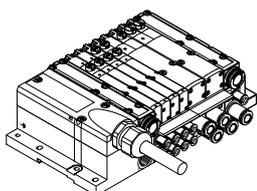
The signals are transmitted from the controller to the valve terminal via a pre-assembled or self-assembled multi-core cable to the multi-pin plug connection. This substantially reduces installation time.
