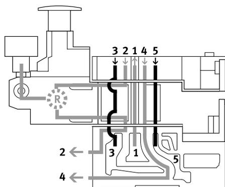
This pressure regulator regulates the pressure in duct 2 after the pressure medium flows through the valve. During exhausting, the air flow in the valve is exhausted from duct 2 to duct 3 via the pressure regulator.
