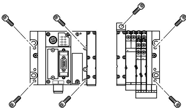
The MPA valve terminal is screwed onto the mounting surface using six M4 or M6 screws. The mounting holes are on the left end plate (CPX) and on the right end plate MPA.
