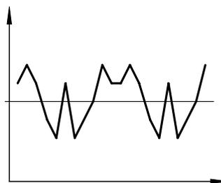
The repetition accuracy is the margin within which the fluidic output variable is scattered when the same electrical input signal coming from the same direction is repeatedly adjusted. The repetition accuracy is expressed as a percentage of the maximum fluidic output signal.
