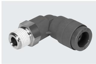
Flame-retardant push-in fitting for use in all areas where there is a risk of fire, for example welding systems in the automotive industry, and in the construction industry. For pneumatic applications with a temperature range up to 60°C and a pressure range up to 10 bar. Tubing O.D. 4, 6, 8, 10 and 12 mm with connecting thread R1/8 ... R1/2 and G1/8 ... G1/2.
