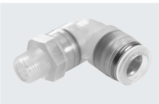
Polypropylene fitting for use in applications with extreme media influences. For pneumatic applications with a temperature range up to 60°C and a pressure range up to 10 bar. Tubing O.D. 4, 6, 8, 10 and 12 mm with connecting threads R1/8 ... R1/2.
