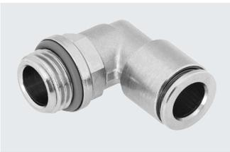
All metal push-in fitting made of chemically nickel-plated brass. High corrosion resistance CRC 3 and chemical resistance. For pneumatic applications with a temperature range up to 150°C and a pressure range up to 20 bar. Tubing O.D. 4, 6, 8, 10, 12 and 14 mm with connecting thread M5, M7 and G1/8 ... G1/2.
