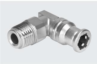
Stainless steel push-in fitting. Maximum corrosion resistance CRC 4 and chemical resistance with approval for use in the food and packaging industry. For pneumatic applications with a temperature range up to 120°C and a pressure range up to 10 bar. Tubing O.D. 4, 6, 8, 10, 12 and 16 mm with connecting threads M5 and R1/8 ... R1/2.
