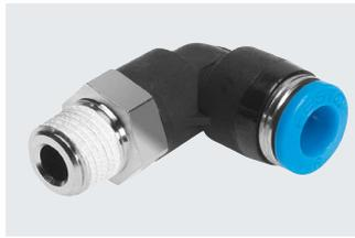
Wide selection of push-in fittings for pneumatic applications with a temperature range up to 80°C and a pressure range up to 14 bar. Tubing O.D. 4, 6, 8, 10, 12, 16 and 22 mm with connecting threads R1/8 ... R1/2 and G1/8 ... G3/4.
