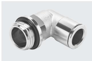
Attractively priced metal push-in fitting for pneumatic applications with a temperature range up to 70°C and a pressure range up to 16 bar. Tubing O.D. 3, 4, 6, 8, 10, 12 and 14 mm with connecting thread M5, M7 and G1/8 ... G1/2.
