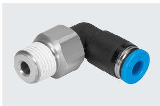
Push-in fitting with swivel joint, rotatable 360°. The ball bearing enables rotating movements in the application up to max. 500 rpm. For pneumatic applications with a temperature range up to 60°C and a pressure range up to 14 bar.
