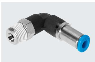
Push-in fitting that blocks the air flow after the tubing is disconnected. For pneumatic applications with a temperature range up to 60°C and a pressure range up to 14 bar.
