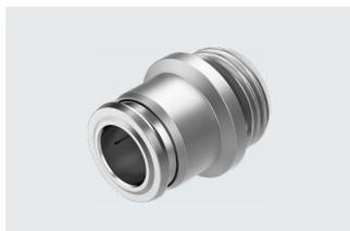
Stainless steel push-in fitting. Maximum corrosion resistance CRC 4 and chemical resistance. For pneumatic applications with a temperature range up to 150°C and a pressure range up to 16 bar. Tubing O.D. 4, 6, 8, 10 and 12 mm with connecting thread M5, M7 and G1/8 ... G1/2.
