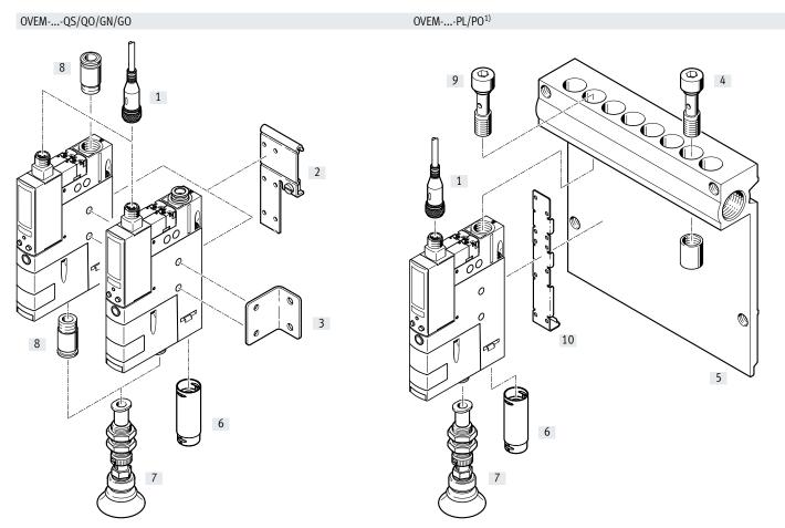
1) Hollow bolt [9] and mounting bracket [10] are included in the scope of delivery for the OVEM-...-PL/PO.
