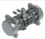
With the single-acting quarter turn actuator, the incoming compressed air moves the pistons in one direction. This generates the torque of the actuator. The springs built into the actuator are pre-tensioned at the same time. This spring force generates the torque in the opposite direction of rotation when the pressure chambers of the actuator are exhausted. This causes the process valve to move to the required initial position.
