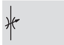
Flow control acting at both sides GRLO/GRGO
