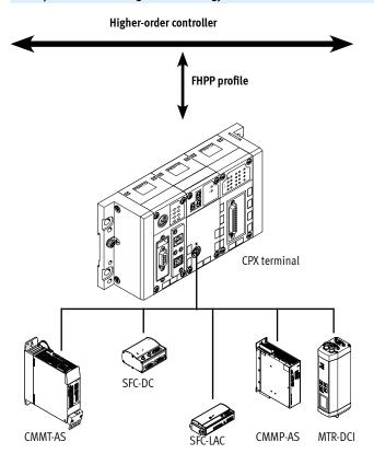
The control block CPX-CM-HPP makes all of Festo's electric drive technology compatible with all industrial communication interfaces.
