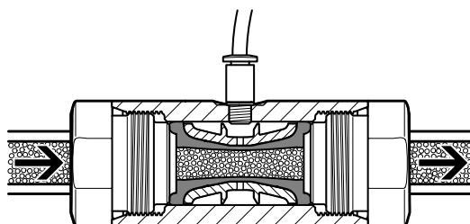
In the normal position, the pinch valve is open. The pinch valve sleeve closes when the valve is pressurised, shutting off the material flow. When pressure is no longer applied, the valve opens due to the inherent stress of the pinch valve sleeve or the pressure of the flow medium. The valve can be used to shut off liquid and powdery media, solids (granules) as well as mixtures of substances.
