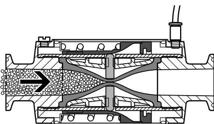
In the normal position, the pinch valve is closed. The pinch valve sleeve opens when the valve is pressurised, releasing the material flow. When pressure is no longer applied, a spring closes the valve. The valve can be used to shut off liquid and gaseous media.
