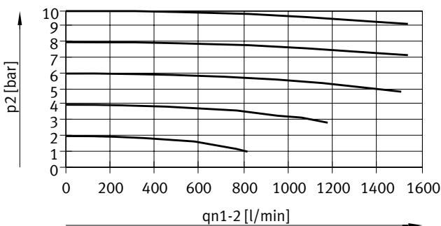
**Flow rate  $q_{n2}$  of 2 → 3 as a function of excess output pressure  $p_2$**
