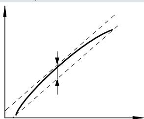
A perfectly linear progression of the control characteristic of the output pressure is theoretical. The maximum percentage deviation from this theoretical control characteristic is referred to as the linearity error. The percentage value refers to the maximum output pressure. (full scale)
