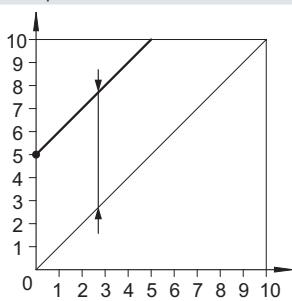
If, for example, a VPPM cannot be exhausted for safety reasons, the minimum pressure can be increased from the zero point. The smallest setpoint value is then assigned an output pressure of 5 bar, for example, and the largest setpoint value an output pressure of 10 bar. Zero point suppression is automatically switched off if the zero point offset is used.
