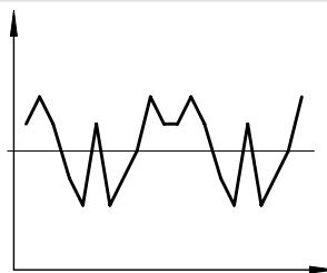
The repetition accuracy is the margin within which the fluid output variables are scattered when the same electrical input signal coming from the same direction is repeatedly adjusted. The repetition accuracy is expressed as a percentage of the maximum fluid output signal.
