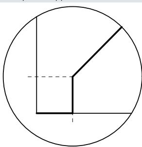
In real-world applications, it is possible for there to be a residual voltage or residual current at the setpoint input of the VPPM via the setpoint generator. Zero point suppression is used so the valve is reliably exhausted at a setpoint value of zero.
