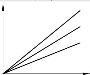
In the delivery status, 100% setpoint value corresponds to 100% of the fluid output signal. Pressure range adaptation or adjustment enables the fluid output variable to be matched to the setpoint value.
