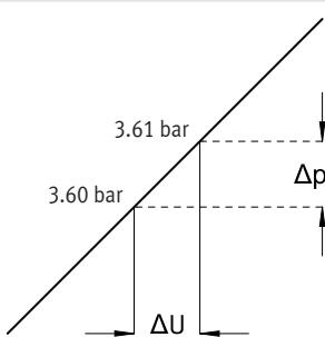
The response sensitivity of the device determines how sensitively one can change, i.e. adjust, a pressure. The smallest setpoint value difference that results in a change in the output pressure is referred to as the response sensitivity.
