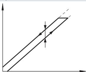
There is always a linear relationship within a certain tolerance between the setpoint value entered and the pressure output. Nevertheless, it makes a difference whether the setpoint value is entered as rising or falling. The difference between the maximum deviations is referred to as hysteresis.
