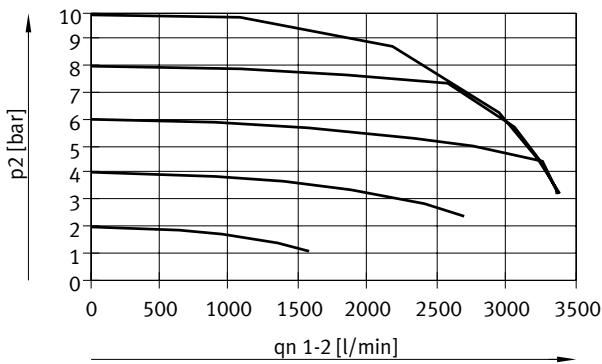
**Flow rate  $q_n$  of 2 → 3 as a function of excess output pressure  $p_2$**
