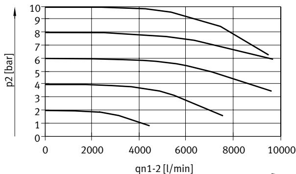
**Flow rate  $q_n$  of 2 → 3 as a function of excess output pressure  $p_2$**
