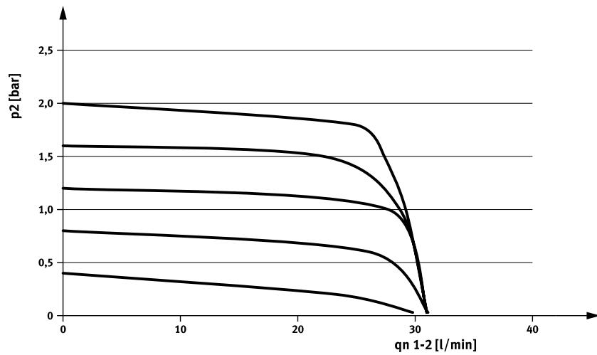
Flow rate  $q_n$  from 2 → 3 as a function of output pressure  $p_2$
