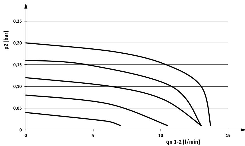
Flow rate  $q_n$  from 2 → 3 as a function of output pressure  $p_2$
