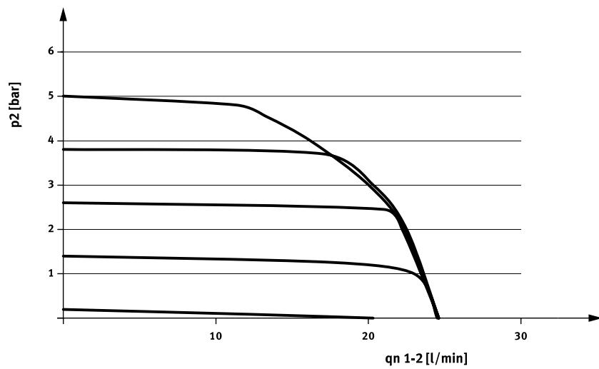
Flow rate  $q_n$  from 2 → 3 as a function of output pressure  $p_2$
