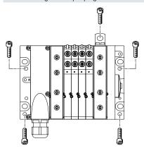
The MPA-L valve terminal is screwed onto the mounting surface using four M4 or M6 screws. The mounting holes are on the multi-pin plug connection and on the right-hand end plate. Optional mounting brackets are also available.
