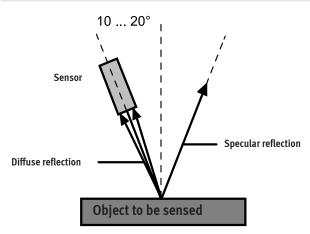
In the case of diffuse sensors with intensity differentiation, diffuse sensors with background suppression and distance and colour sensors, sensing is based on diffuse reflection. These sensors therefore require as much diffuse reflection as possible. Total reflection makes detection difficult and must therefore be avoided. The type of reflection is not relevant for retro-reflective sensors and through-beam sensors.
