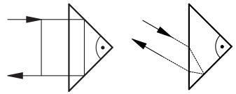
Small optical structures (mini/micro) are very well suited for laser sensors, but have the disadvantage that they reflect slightly less light and therefore have a smaller detection range.
