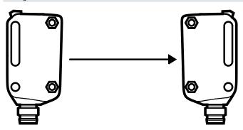
In the case of through-beam sensors, the transmitter and receiver are located in different housings, which must be installed opposite one another. Each object that interrupts the light beam between the transmitter and the receiver is detected. This is one of the most reliable principles in harsh environmental conditions. The disadvantage is that two separate components (transmitter and receiver) have to be wired and set up.
