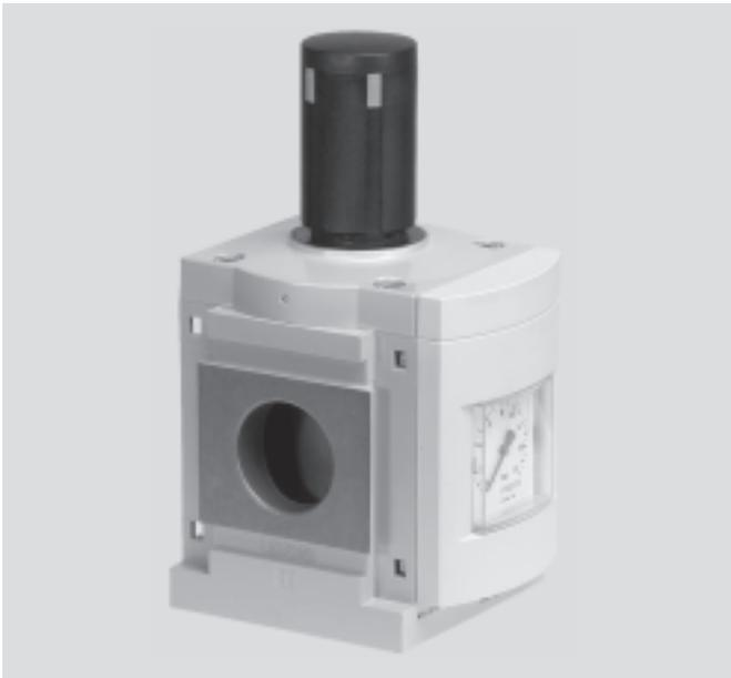
The pressure regulator maintains a constant working pressure (secondary side), regardless of the pressure variations in the system (primary side) and the air consumption.
