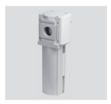
Fine and micro filters, with 1 micron or 0.01 micron filtration grades, remove submicronic water or oil droplets and dirt particles for exceptionally clean compressed air.
