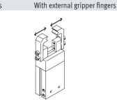
The indicated opening and closing times [ms] have been measured at room temperature and 6 bar operating pressure without additional gripper fingers. The grippers must be throttled for larger masses [g]. Opening and closing times must then be adjusted accordingly.
