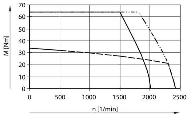
Winding HV (without/with brake)
