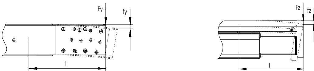
$F_y/F_z$  at which the characteristic curves were determined
