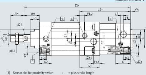
[1] Socket head screw with female thread for mounting components
