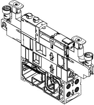
Additional functions can be added to each valve position between the sub-base (manifold sub-base) and the valve.
