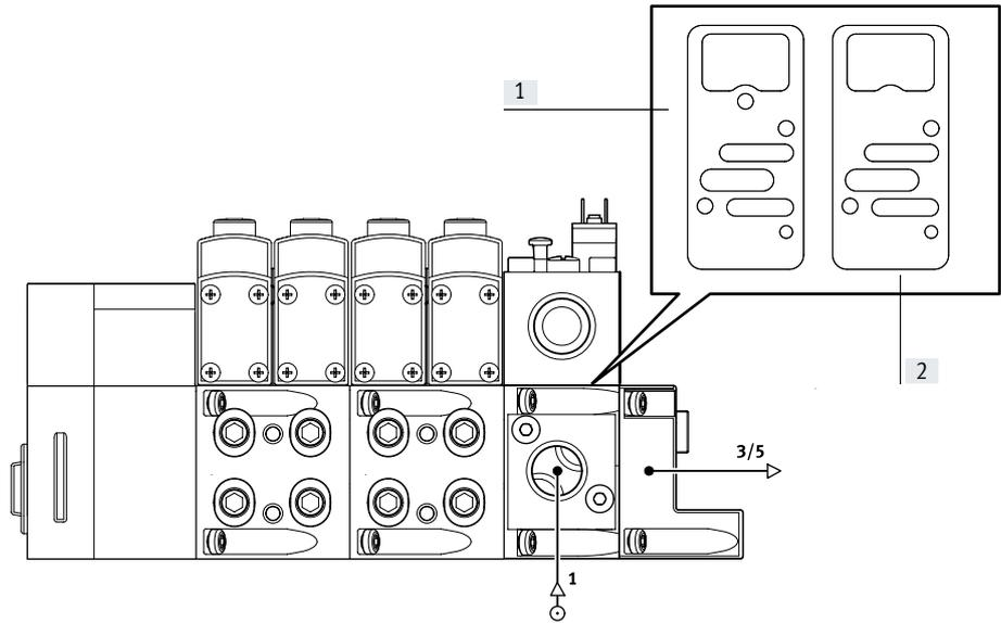
[1] Seal for internal pilot air supply
