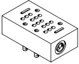
Intermediate plate with integrated exhaust air flow controls at ports 3 and 5 for regulating cylinder speed
