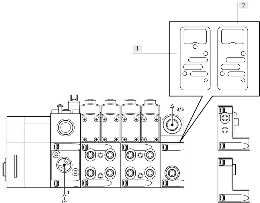
[1] Seal for internal pilot air supply
