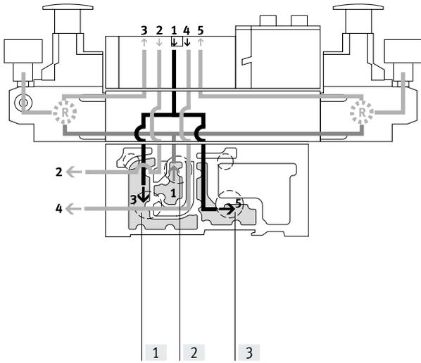
With this pressure regulator, the supply air (duct 1) is split and routed directly to both pressure regulators. In each case the regulated supply air is present in ducts 3 and 5 on the valve. The valve is thus operated in reversible mode.
