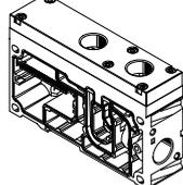
Supply plates for VTSA/VTSA-F, exhaust port 3/5 common
