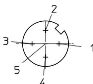
[1] Connector plug M12x1, 5-pin
