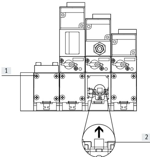
[1] Loosen the retaining screws in the covering
