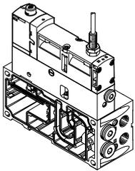
The pilot air switching valve is a combination of a 5/2-way solenoid valve with switching position sensing and the intermediate plate VABF-S4-...-S. It enables verifiable switching on and off (sensing function) of the pilot air supply from duct 1 to 14 for the entire pressure zone or valve terminal.
