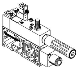
The soft-start valve is separately electrically actuated, independently of the multi-pin plug connection, AS-Interface or fieldbus interface, via a square plug of type C to EN 175301-803 or optionally via an M12 adapter.
