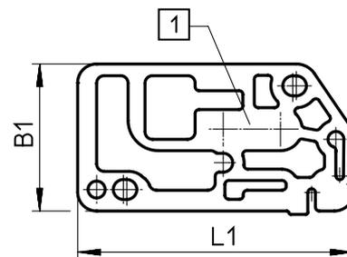
[1] With elongated hole, internal pilot air supply
