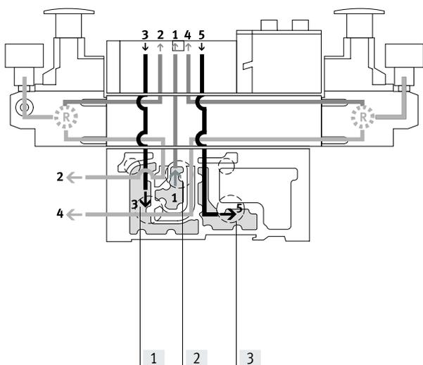
This pressure regulator regulates the pressure in ducts 2 and 4 after the pressure medium flows through the valve.
