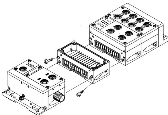
The mechanical connection between the CPX modules in metal design is created using special angle fixings. The CPX terminal can thus be expanded at any time.
