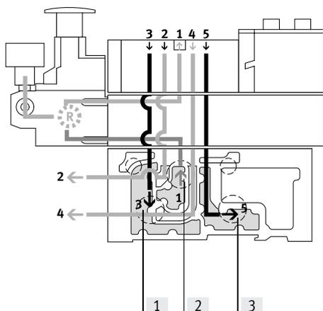
This pressure regulator regulates the pressure upstream of the valve in duct 1. Ducts 2 and 4 thus have the same regulated pressure.
