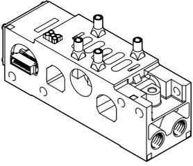
Adaptation to size 65 mm ISO size 3 is based on a modular system which consists of manifold sub-bases and valves. The manifold sub-bases contain a duct seal and an electrical link, are screwed together and thus form the support system for the valves.
