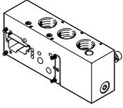
The adapter plate VABA... is used for adapting valves of width 65 mm ISO size 3 to valve terminal VTSA/VTSA-F. Ports for supply/exhaust air and pilot air supply are available.
