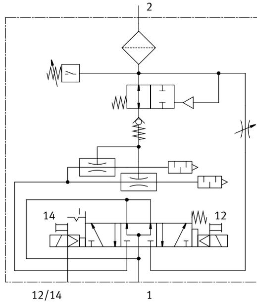
The vacuum generator is supplied internally via duct 1 of the manifold sub-base of the valve terminal.
