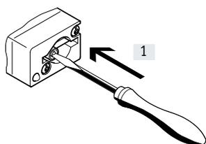
[1] Press in the plunger of the manual override using a pointed object or screwdriver. The valve is in the switching position.
