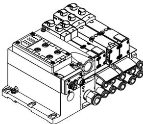
A special feature of the AS-Interface is the simultaneous transmission of data and supply power via a two-wire cable. The encoded cable profile prevents connection with reverse polarity. The valve terminal with AS-Interface is available in the following versions:
