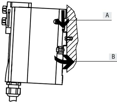
The valve terminal VTSA/VTSA-F/VTSA-F-CB is hooked onto the H-rail (see arrow A).
