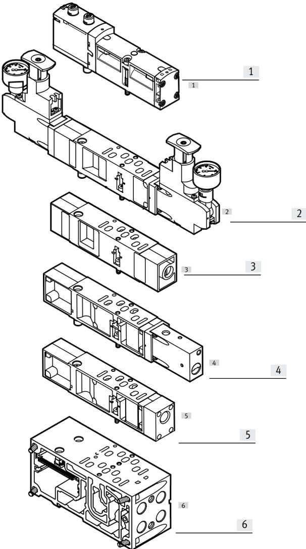
The following component sequence is recommended for valve positions with vertical stacking:
