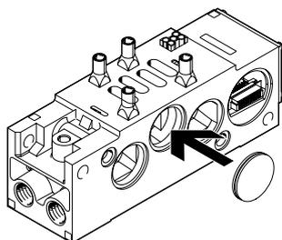
It is possible to have different supply pressures in the area containing valves with a width of 65 mm by installing isolating discs between two manifold blocks. It should be noted that the isolating disc is inserted into the manifold sub-base from the right.
