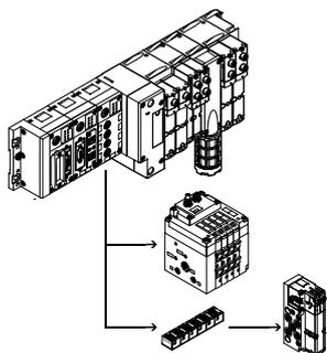
The optional CP string extension enables additional valve terminals and I/O modules to be connected to the bus node of the CPX terminal on up to 4 CP strings. Different input and output modules as well as valve terminals MPA-S and CPV can be connected.
