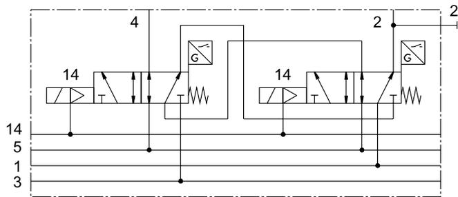
For the control block with safety function VOFA-B26-T52-... for the valve terminal, two 5/2-way solenoid valves of width 26 mm are pneumatically linked via two ducts, using an intermediate plate as vertical stacking element (output 2 is switched in parallel, output 4 is switched in series).
