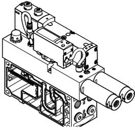
5/3-way solenoid valve, with switching position 12 retained.
