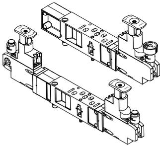
An adjustable pressure regulator can be installed between the base plate (manifold sub-base) and the valve in order to control the force of the triggered actuator.
