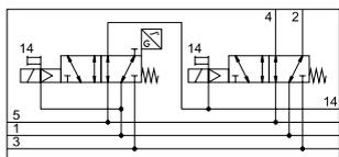
The function for switching off the pilot air is essentially achieved by combining the intermediate plate type VABF-S4-...-S with the 5/2-way single solenoid valve type VSVA-B-M52-MZD-...-1T1L-APX-0.5.
