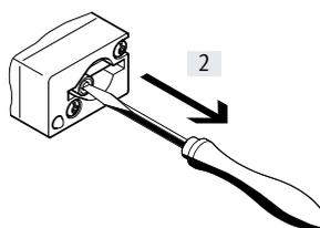
[2] Remove the pointed object or screwdriver. The spring force pushes the plunger of the manual override back. Valve returns to its initial position (not with double solenoid valve, code J, D).
