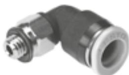
Miniature push-in fittings for maximum component density in confined spaces. For pneumatic applications with a temperature range up to 80°C and a pressure range up to 14 bar. Tubing O.D. of 2, 3, 4 and 6 mm with connecting threads M3, M5, M6, M7, R1/8 and G1/8.
