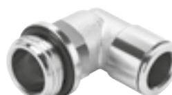
Attractively priced metal push-in fitting for pneumatic applications with a temperature range up to 70°C and a pressure range up to 16 bar. Tubing O.D. 3, 4, 6, 8, 10, 12 and 14 mm with connecting thread M5, M7 and G1/8 ... G1/2.
