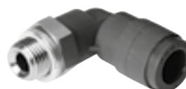
Flame-retardant push-in fitting for use in all areas where there is a risk of fire, for example welding systems in the automotive industry, and in the construction industry. For pneumatic applications with a temperature range up to 60°C and a pressure range up to 10 bar. Tubing O.D. 4, 6, 8, 10 and 12 mm with connecting thread R1/8 ... R1/2 and G1/8 ... G1/2.
