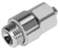
Stainless steel fitting for use in areas subject to intensive cleaning. Maximum level of corrosion resistance CRC 4. For pneumatic applications with a temperature range up to 120°C and a pressure range up to 12 bar.
