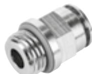
All metal push-in fitting made of chemically nickel-plated brass. High corrosion resistance CRC 3 and chemical resistance. For pneumatic applications with a temperature range up to 150°C and a pressure range up to 20 bar. Tubing O.D. 4, 6, 8, 10, 12 and 14 mm with connecting thread M5, M7 and G1/8 ... G1/2.
