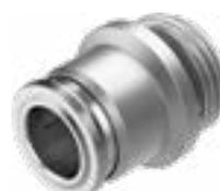
Stainless steel push-in fitting. Maximum corrosion resistance CRC 4 and chemical resistance. For pneumatic applications with a temperature range up to 150°C and a pressure range up to 16 bar. Tubing O.D. 4, 6, 8, 10, 12, 14 and 16 mm with connecting thread M5, M7 and G1/8 ... G1/2.
