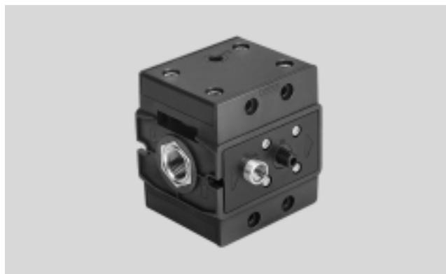
Pneumatically actuated soft start valve for gradual pressure build-up in pneumatic systems. This ensures safe start-up of pneumatic systems. A minimal amount of air flows into the system via an adjustable flow control valve. Output pressure is built up slowly. Downstream cylinders and
