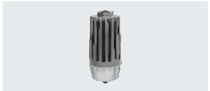
The filter silencer cleans the collected exhaust air from pneumatic control systems. The exhaust air escapes into the atmosphere via a fine filter insert (filter efficiency > 99.99%).
