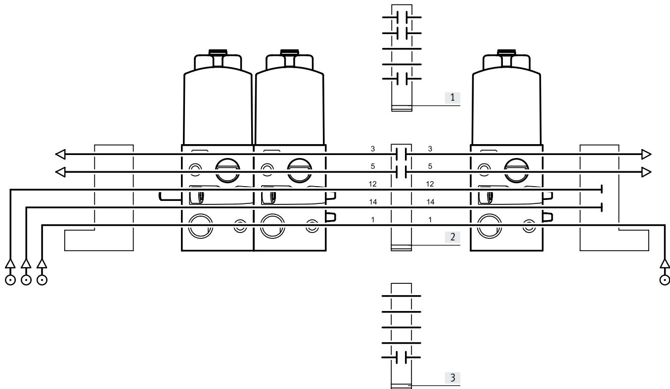
[1] Pressure zone separation in ducts 1, 3 and 5. Pressure supply and exhausting via the respective end plate for each of the two pressure zones. Pilot air is supplied jointly via the left end plate.
