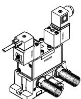
The directional control valve has a pilot control to ISO 15218. The solenoid coil plugged onto the armature tube can be chosen in different designs and operating voltages.
