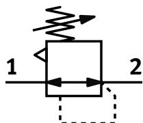
The pressure regulator enables a particular pressure in the regulated port to be set manually upstream or downstream of the valve.
