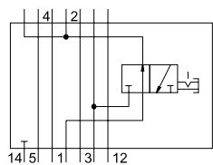
Vertical pressure shut-off plate for blocking duct 1 and duct 14 upstream of a valve.
