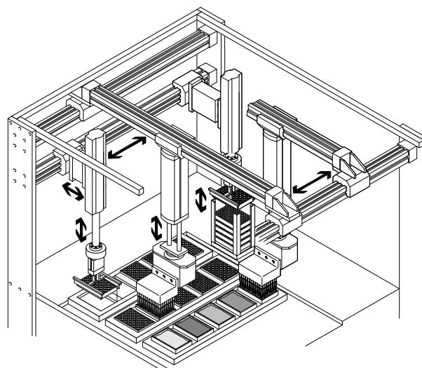
Feeding workpieces with simultaneous quality inspection via a vision system
