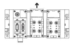
For longer valve terminals, there is an additional mounting bracket (for the CPX terminal) that can be fitted in any module.
