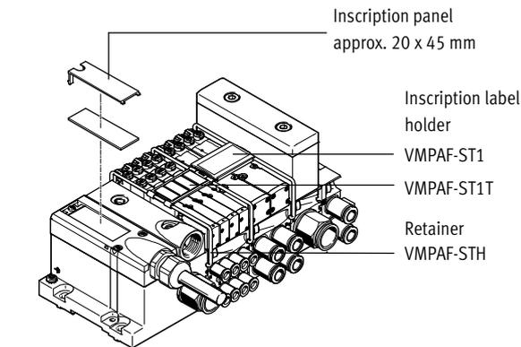
An inscription label holder VMPAF-ST1 (Part No. 546 228, code T in the order code, for holding paper labels) or VMPAF-ST1T (Part No. 544 422, for holding IBS-9x20 inscription labels) can be mounted on each manifold rail for labelling the valves.
