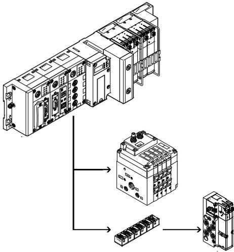
The optional string extension enables additional valve terminals and I/O modules to be connected to the fieldbus node of the CPX terminal. Different input and output modules as well as valve terminals can be connected.
