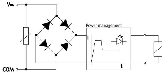
Each MPA solenoid coil is protected with a spark arresting protective circuit as well as against polarity reversal. All valve types are additionally equipped with integrated current reduction.
