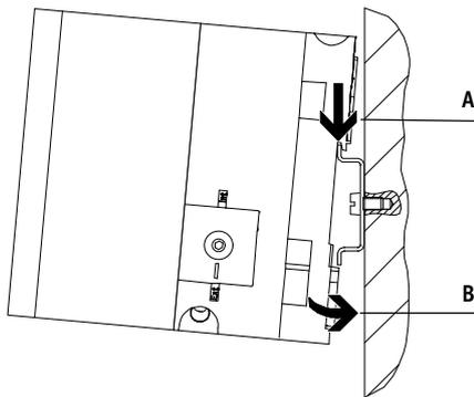
The MPA-F valve terminal is attached to the H-rail (see arrow A). The valve terminal MPA-F is then swivelled onto the H-rail and secured in place with the clamping components (see arrow B).
