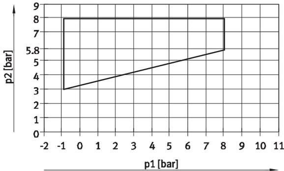
For valves in width 20 mm with code: MS, NS, KS, HS, DS
