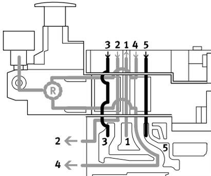
This pressure regulator regulates the pressure in duct 4 after the pressure medium flows through the valve. During venting, the exhaust flow in the valve is from duct 4 to duct 5 via the pressure regulator.
