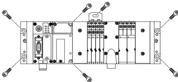
The MPA-F valve terminal is screwed onto the mounting surface using six M6 screws. The mounting holes are on the left-hand end plate (CPX) and on the right-hand end plate (MPA-F).
