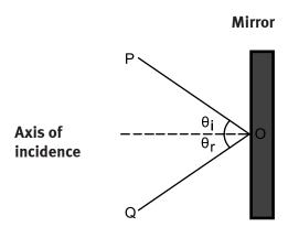
Specular reflection is the perfect reflection of light (or other kinds of wave) from a surface, when incident light from a single direction is reflected in a single direction.
