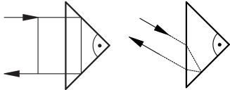
Small optical structures (mini/micro) are very well suited for laser sensors, but have the disadvantage that they reflect slightly less light and therefore have a smaller detection range.
