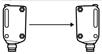
In the case of through-beam sensors, the transmitter and receiver are located in different housings, which must be installed opposite one another. Each object that interrupts the light beam between the transmitter and the receiver is detected. This is one of the most reliable principles in harsh environmental conditions. The disadvantage is that two separate components (transmitter and receiver) have to be wired and set up.
