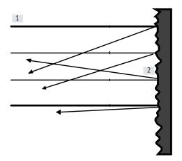
Diffuse reflection is the reflection of light from an uneven or grained surface when an incident beam is reflected at many different angles.
