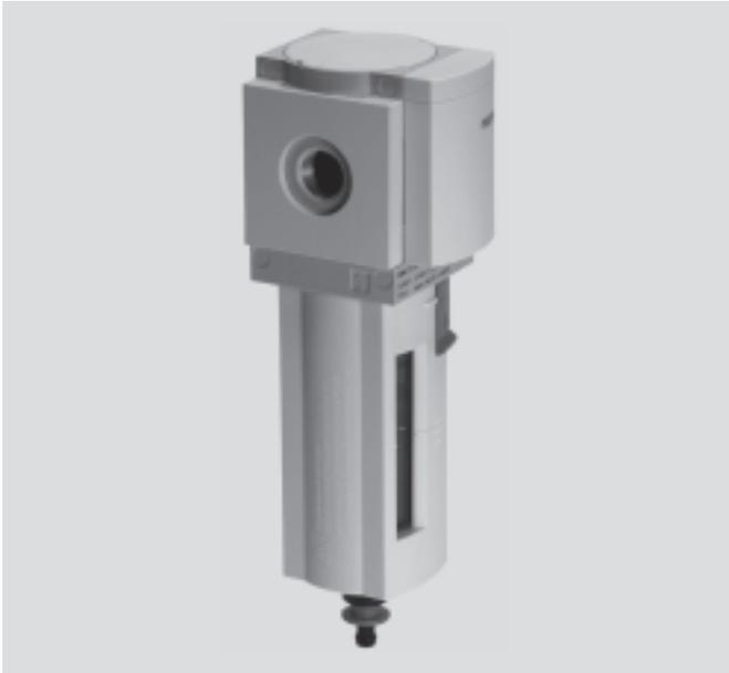
Fine and micro filters, with 1 micron or 0.01 micron filtration grades, remove submicronic water or oil droplets and dirt particles for exceptionally clean compressed air.
