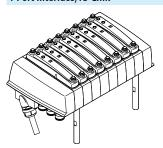
I-Port/IO-Link® consists of a central master and the I-Port interface/IO-Link devices connected by special connecting cables. This permits a decentralised layout of the devices.
