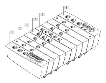
[1] Left end plate with electrical connection (multi-pin or I-Port interface/IO-Link) and pneumatic ports 1, 3 and 5
