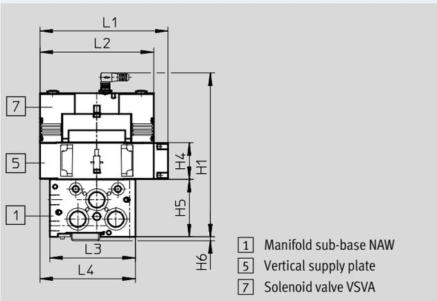
Width 18 mm with manifold sub-base and solenoid valve with pilot interface to ISO 15218
