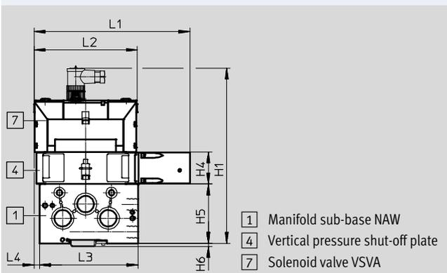
Width 26 mm with manifold sub-base and solenoid valve with pilot interface to ISO 15218
