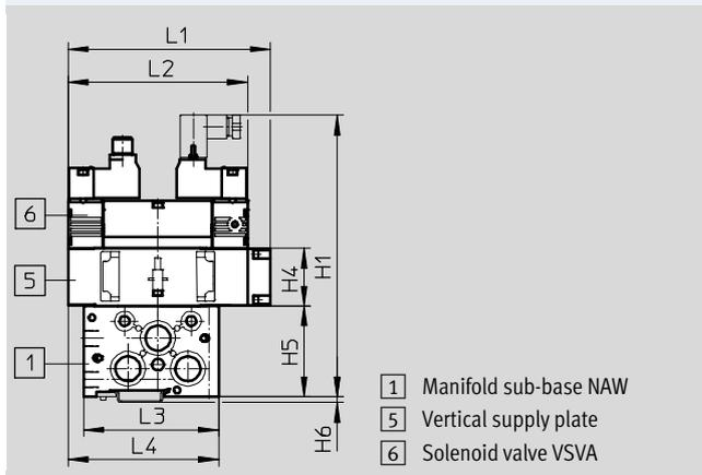
Width 26 mm with manifold sub-base and solenoid valve with central plug
