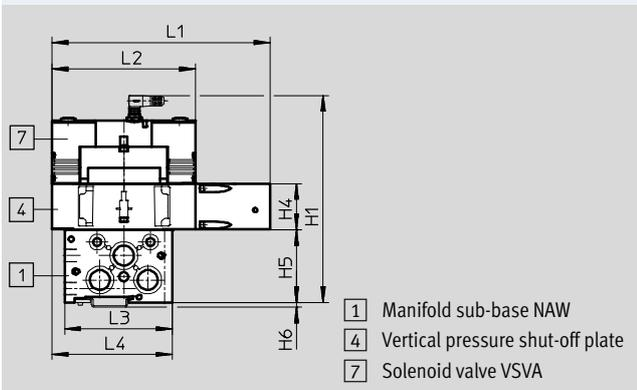
Width 18 mm with manifold sub-base and solenoid valve with pilot interface to ISO 15218
