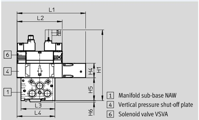
Width 26 mm with manifold sub-base and solenoid valve with central plug
