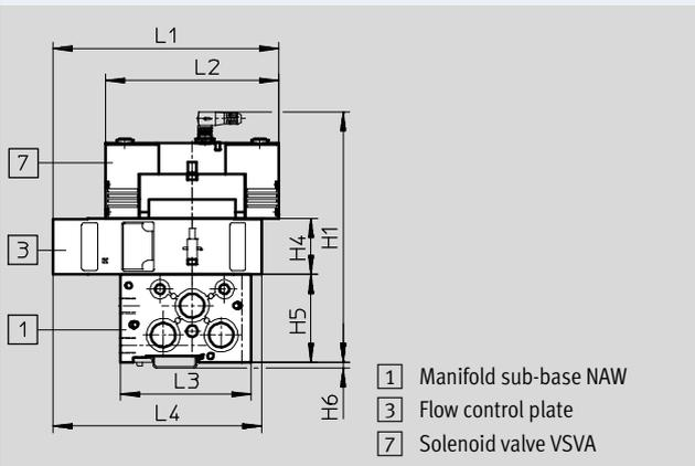
Width 18 mm with manifold sub-base and solenoid valve with pilot interface to ISO 15218
