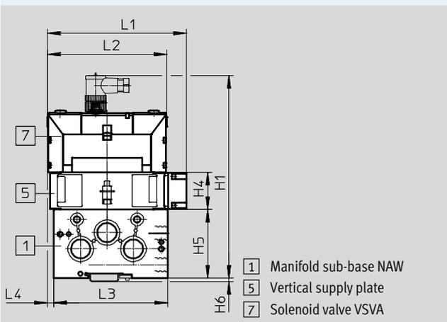
Width 26 mm with manifold sub-base and solenoid valve with pilot interface to ISO 15218
