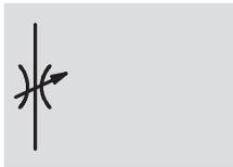
Flow control valve, operative in both directions
