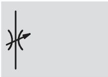
Flow control valve, operative in both directions
